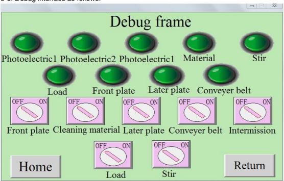
This interface are all for test switch, it is for us to test machine function and action before delivery.
