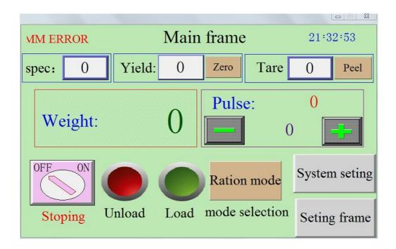
The ERROR (left up corner) means the machine was failure warning.
