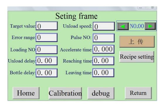
Target value: in condition of automatic mode and fine tuning mode, the specification size of packing powder can be adjusted automatically by PLC against the powder filling quantity.
