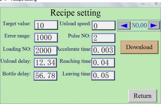
The parameter of this interface is parameter in touch screen, it is not the current running parameter, you can download into PLC.
